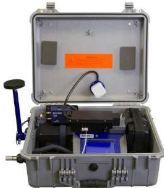
Figure 4.5.2 Dust Trak Aerosol monitor (8533 model) installed in Environmental Enclosure 8535
