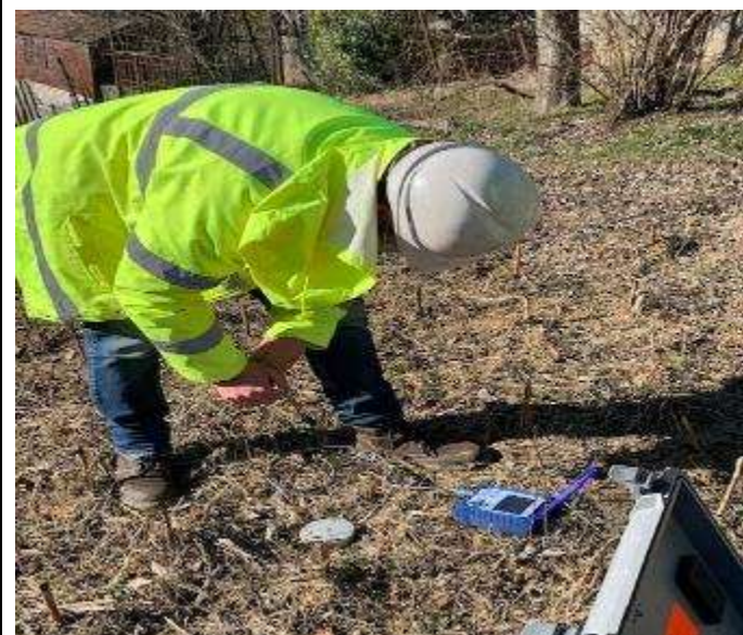
Vibration Monitoring being carried out at the site during reporting period
